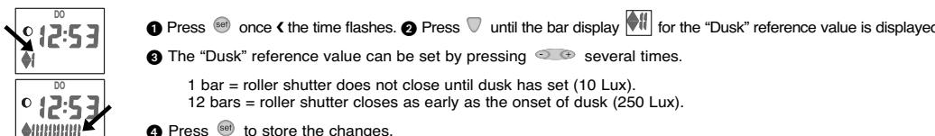
**Tip:** It is best to enter data when the evening dusk reaches the brightness level at which you wish to have the shutter close automatically in the future. To do this, set the "Dusk" reference value to 1 bar, and then press Plus (+) until the moon symbol (O) is displayed. This value then corresponds to the current dusk setting.
