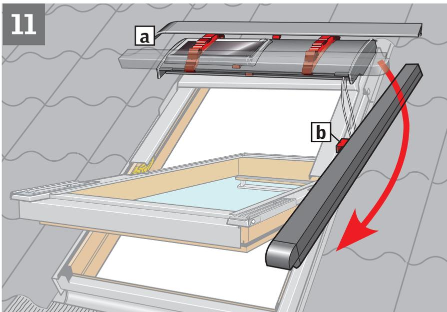
**ENGLISH:** Disengage the first side channel from the transit brackets [a], turn and hold parallel to side frame. Do **not** remove the transit device [b] at this stage.
