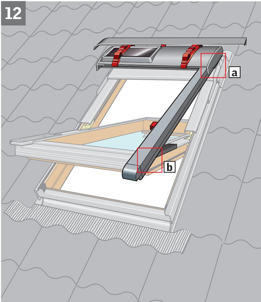
**ENGLISH:** Pull side channel downwards. **It is necessary to pull the side channel hard.** Lift the awning top cover and slide the side channel straight into the groove in the top cover. Ensure that the cords do not cross each other and that they are positioned in the side channel **[a]**. Snap sliding device **[c]** onto the bottom bracket **[b]**.
