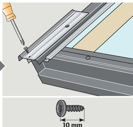
**ENGLISH:** Remove and discard cover screws [a](#). Place sealant on screw holes. Fix bottom brackets with 45 mm screws supplied [b](#) and adjust so that they are parallel to the cover. Drill hole in cover through hole in bracket and fix bracket with 10 mm screw supplied [c](#).
