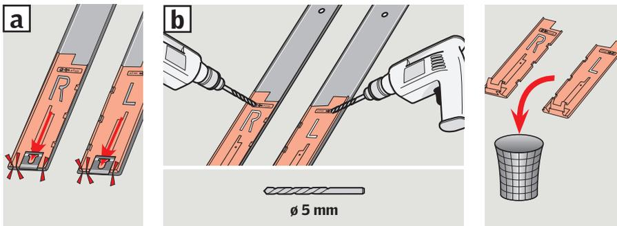
**ENGLISH:** Fit distance sheets (**R** and **L**) on the underside of the covers. Slide the sheets completely down into the cover brackets **a**. Drill holes, through the covers, at the marks using a  $\varnothing$  5 mm drill **b**.
