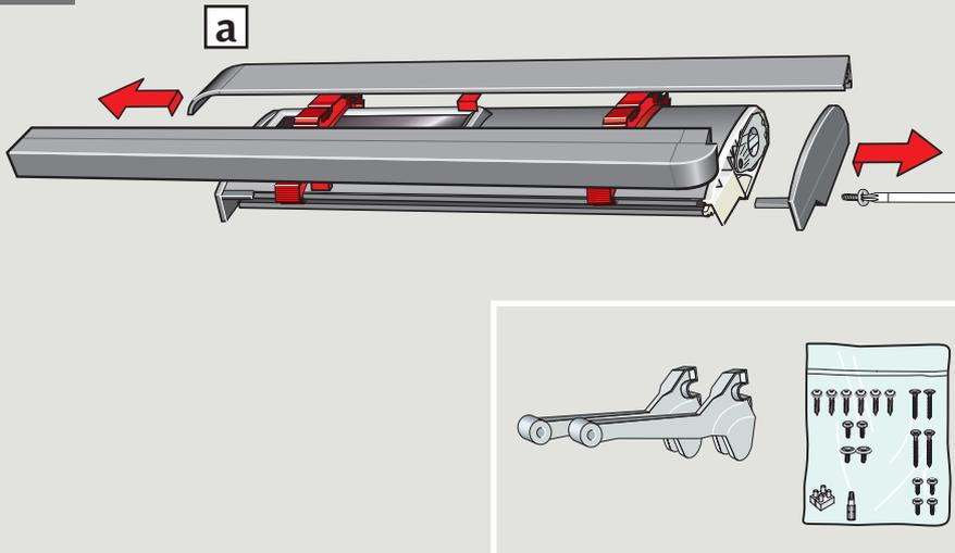
**ENGLISH:** Remove plastic covers from both sides **a**. Place adaptor on axle and turn into position **b**. Fix adaptor with screw supplied **c**. Refit plastic covers **d**.
