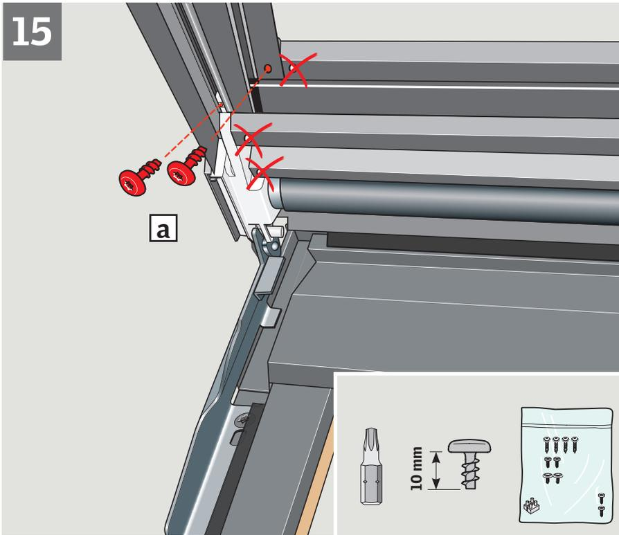
**ENGLISH:** Fix side channels with screws supplied [a]. Remove and discard transit brackets and devices [b].
