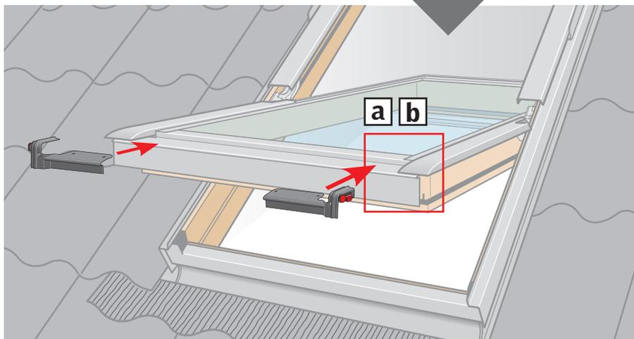
**ENGLISH:** Position bottom brackets temporarily on bottom sash and drill holes for screws. Remove brackets and place sealant on screw holes **a**. Position bottom brackets and fit with screws supplied. Remove transit device **b**.
