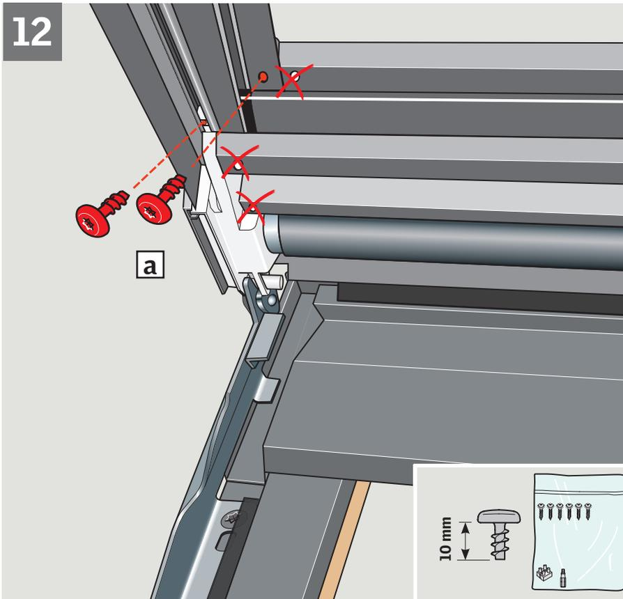
**ENGLISH:** Fix side channels with screws supplied [a]. Remove and discard transit brackets and devices [b].
