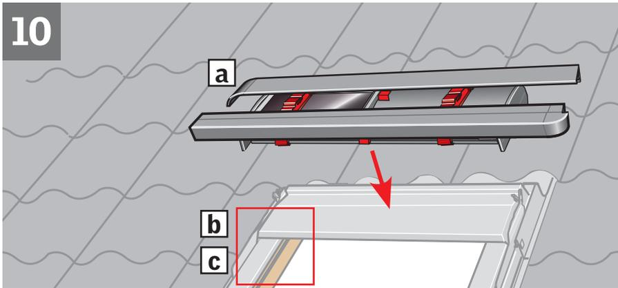
**ENGLISH:** Position awning blind [a]. Fit the awning blind into the bracket and lock it in place [b]. Ensure that the locking bracket is pressed fully home [c].
