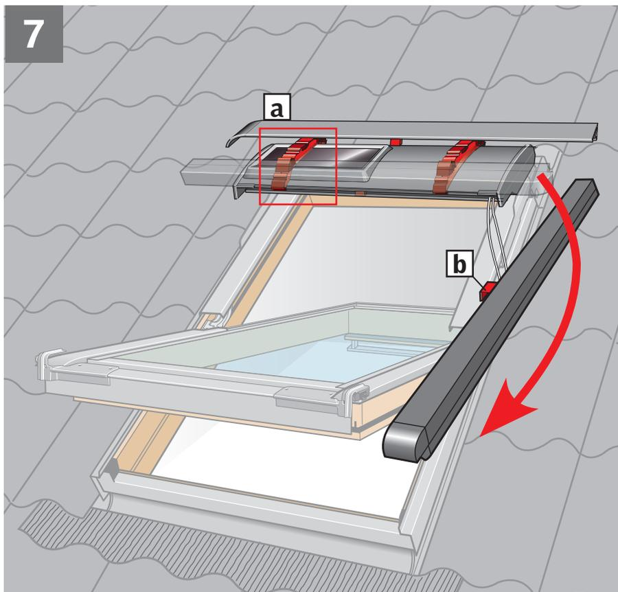
**ENGLISH:** Disengage the first side channel from the transit brackets **[a]**, turn and hold parallel to side frame. Do **not** remove the transit device **[b]** at this stage.
