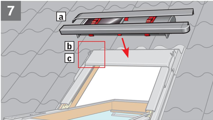
**ENGLISH:** Position awning blind **[a]**. Fit the awning blind into the bracket and lock it in place **[b]**. Ensure that the locking bracket is pressed fully home **[c]**.
