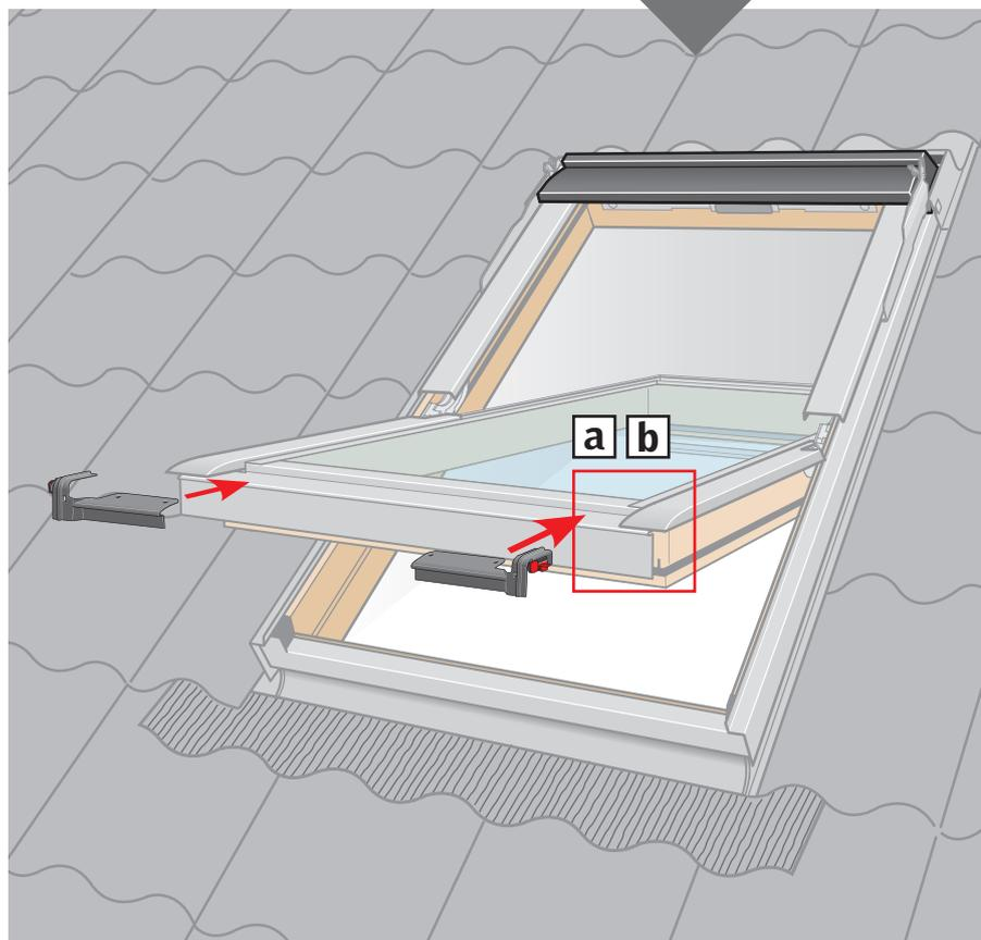
**ENGLISH:** Position bottom brackets temporarily on bottom sash. Drill a pilot hole for screw with a  $\varnothing 3$  mm drill bit and make a mark with bradawl through the other hole. Remove brackets and place sealant on screw holes [a]. Position bottom brackets and fit with screws supplied. Remove transit device [b].
