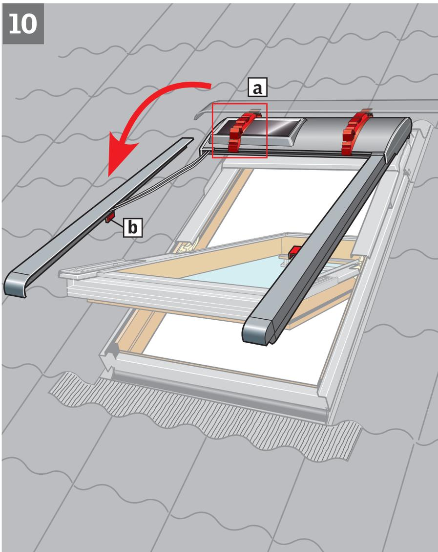
**ENGLISH:** Disengage the second side channel from the transit brackets **a**, turn and hold parallel to side frame. Do **not** remove the transit device **b** at this stage.
