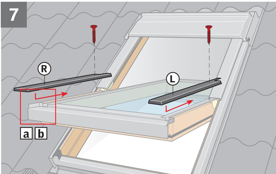
**ENGLISH:** Refit the covers **a**, then drill hole, in sash, through the covers using a  $\varnothing$  3 mm drill **b**.
