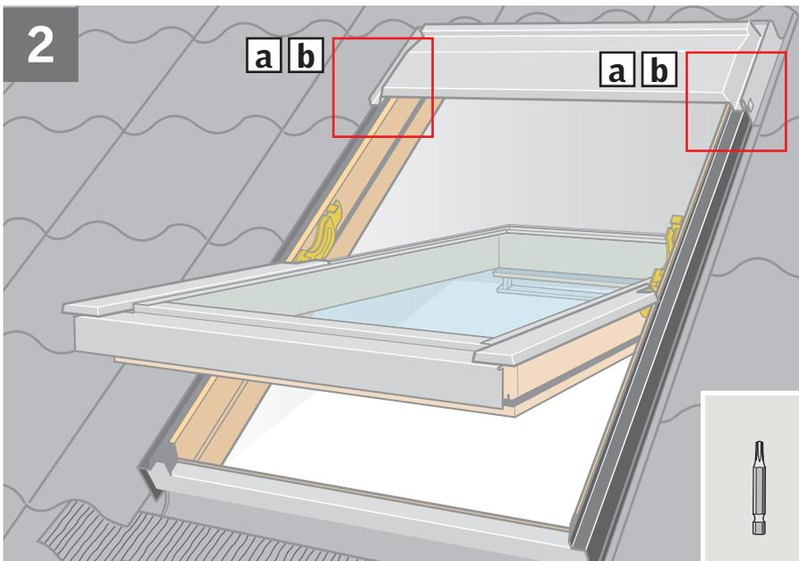
**ENGLISH:** Remove cover screws except the top cover screw [a]. If there is a mark at the top instead of a screw, drill hole through mark [b]. Place sealant on **all** screw holes [c].
