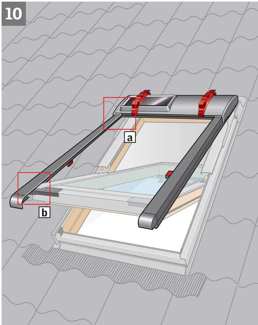
**ENGLISH:** Pull side channel downwards. **It is necessary to pull the side channel hard.** Lift the awning top cover and slide the side channel straight into the groove in the top cover. Ensure that the cords do not cross each other and that they are positioned in the side channel **a**. Snap sliding device **c** onto the bottom bracket **b**.
