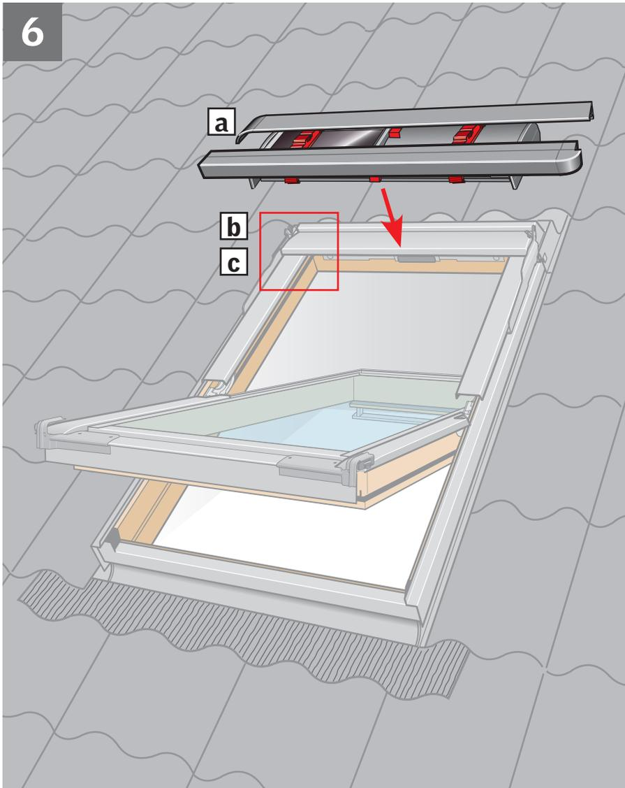
**ENGLISH:** Position awning blind **[a]**. Fit the awning blind into the bracket and lock it in place **[b]**. Ensure that the locking bracket is pressed fully home **[c]**.
