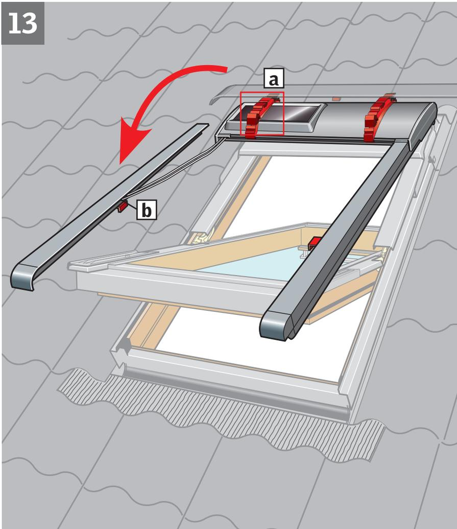
**ENGLISH:** Disengage the second side channel from the transit brackets **a**, turn and hold parallel to side frame. Do **not** remove the transit device **b** at this stage.
