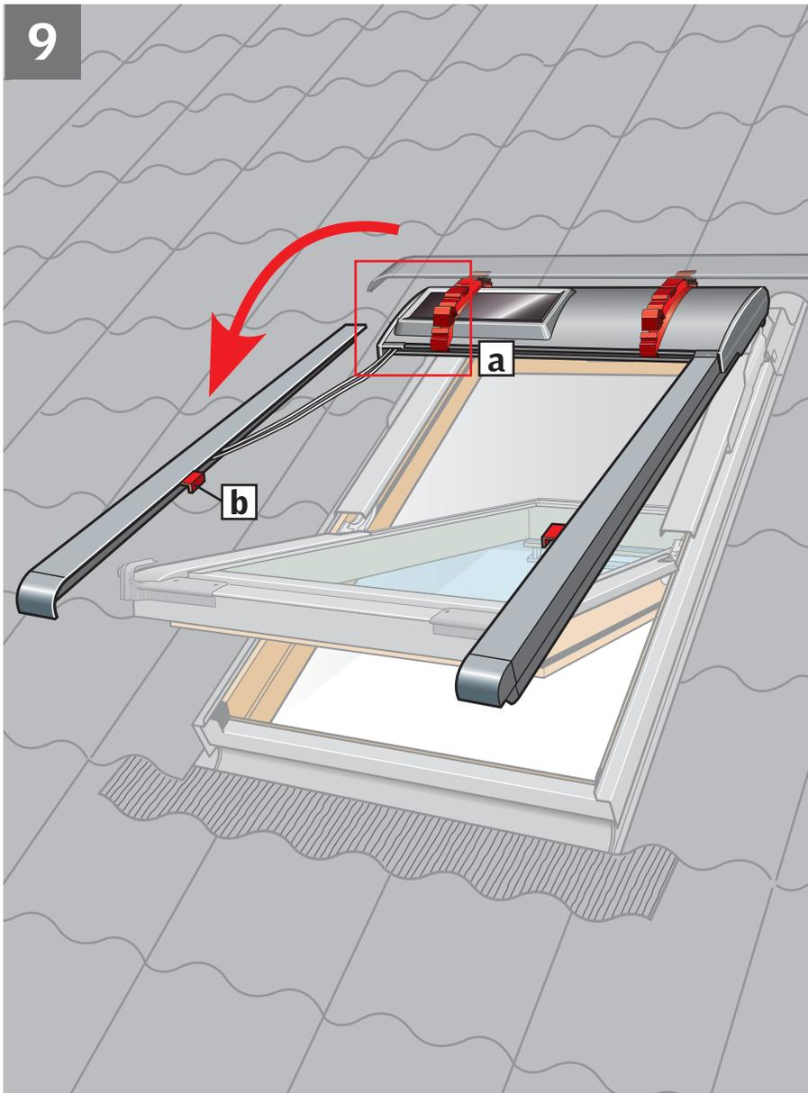
**ENGLISH:** Disengage the second side channel from the transit brackets **a**, turn and hold parallel to side frame. Do **not** remove the transit device **b** at this stage.
